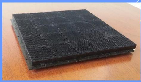
Test load assembled at UdeC with small TK tiles
